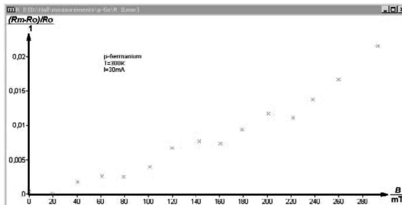
Figure 5: The resistance depending on magnetic field
